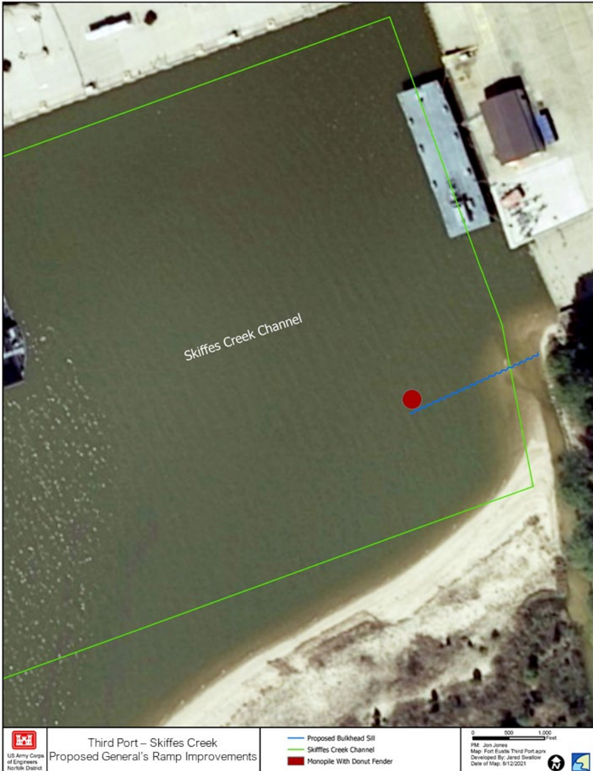
Figure 7. Proposed improvements to the general's ramp area.
